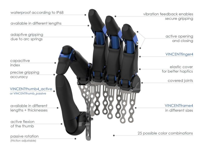
higher grasping force | anatomical design | single finger control unique scope of functions | simple control of all grasps high-strength lightweight constructions
