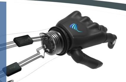
The VINCENTemg2 is currently the smallest digital surface electrode for measuring muscle action potentials for the control of myoelectric prostheses, with two channels.
