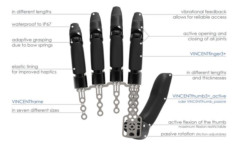
higher grasping force | anatomical design | Single Finger Control unique functionality | easy control of all grasps | high-strength lightweight construction
